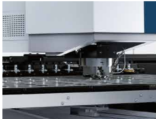
The punching head can rotate any tool to any desired position.
