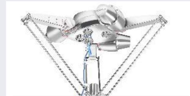
KR DELTA Hygienic robot: designed for use in highly sensitive conditions
