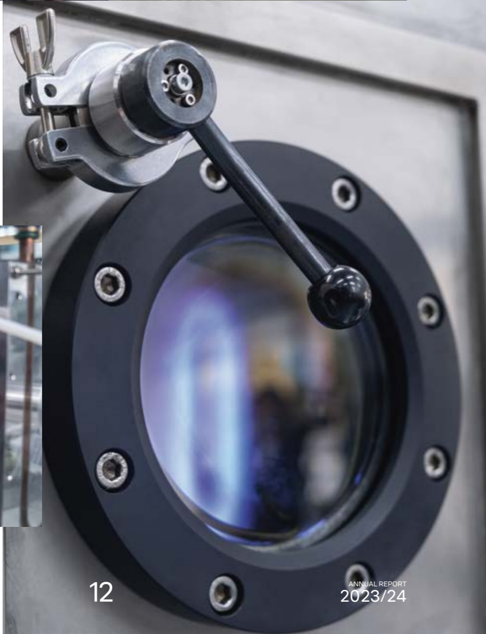
The chambers in the TRUMPF laboratories initialize plasma for various applications. The color of the glow depends on the gas used.
