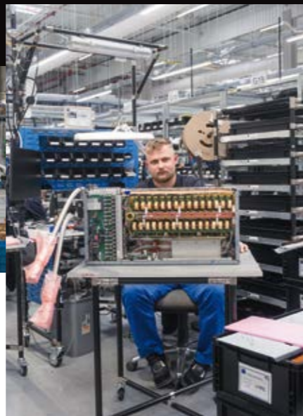
Special generators for every application: Generators for the semiconductor industry are created in Targówek from numerous components some of which are manufactured automatically.
